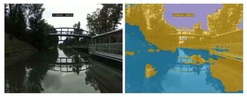
• State-of-the-art fails with false detections on glitter and mirroring
