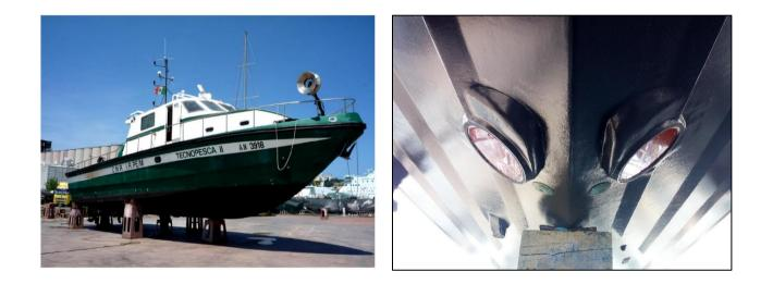
The EM2040 system is a dual head large swath coverage [140-200°] shallow water multibeam echo sounder mounted on the keel of R/V Tecnopesca II with operating frequency range 200-400 kHz. For the water column survey, an optimized frequency between 250 and 300 kHz was used.
