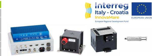
Single components of MBES installation, from left to right: sonar head, I2NS, MRU, mini SVP
